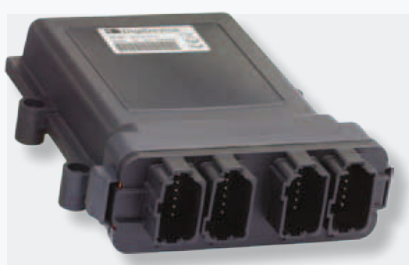
BIG-BLOCK Up to 16 Outputs (PWM) Up to 16 Inputs
